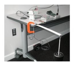
Calibrate a cantilever beam weigh scale and calculate the shunt cal resistor equivalent force value.
