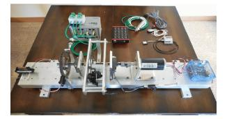
This small motor dynamometer is used as a data acquisition platform for students to connect sensors to different data acquisition systems and record and analyze results in real time.
