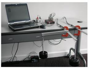
Measure rosette strain gage responses from beams under combined loads and calculate the resulting multiaxial stresses.
